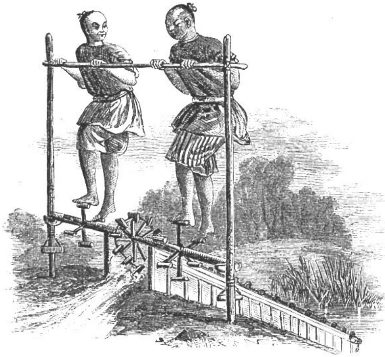
Irrigation by means of an endless chain-pump
